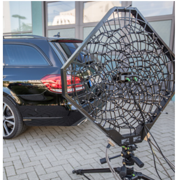
Fibonacci array measurement set up
