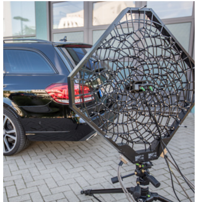
Fibonacci array measurement set up
